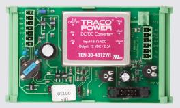
The gateway for connecting of base radio station provides interfacing between a base radio station and digital Armtel DCN and IPN systems. The gateway enables to connect base radio stations such as MOTOROLA GM340 and GM360 or similar to analogue interfaces of the above mentioned systems for communicating with radio network subscribers. The gateway is located near a base FM-radio station or mounted in telecom cabinets or racks, control rooms or office premises.
